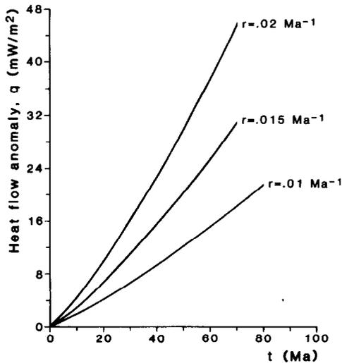
Fig. 11. The surface heat flow for solid-state stretching with constant temperature at the LAB.  $q_m = 20 \text{ mW/m}^2$ . Initial lithospheric thickness = 100 km.
