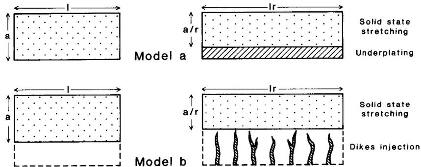
Fig. 7. Two different models of the lithospheric stretching. In model (a), underplating, magma is accreting and solidifying at the base of the lithosphere. In model (b), stretching and injection, extension takes place by solid-state stretching in the upper part of the lithosphere and by dike injection in the lower part.
