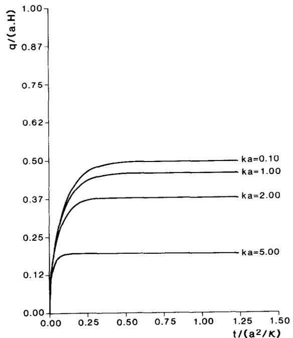
Fig. 6. The heat flow perturbation caused by magma injection when the temperature is constant at the lower boundary.  $(a-b)/a = 1.00$ . All the conventions are the same as above.
