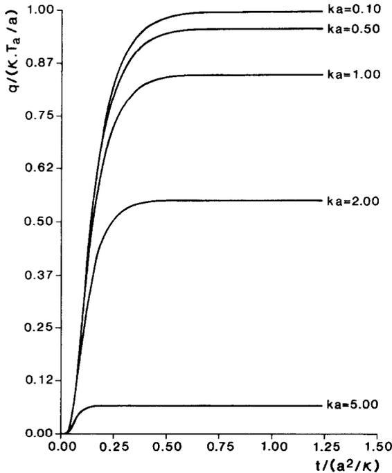
Fig. 3. The surface heat flow at time  $t$  after a stepwise change in temperature at the lower boundary for different dimensionless wavenumbers. The heat flow unit is the amplitude of the heat flow perturbation at the lower boundary; all the other conventions are the same as used in Fig. 2.
