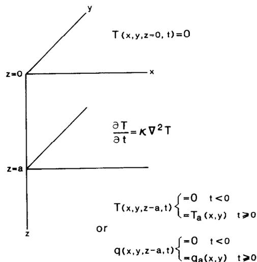
Fig. 1. The geometry, equations, and boundary conditions for the conductive heating model.
