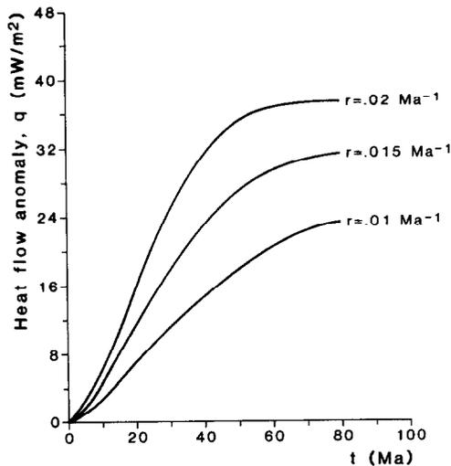
Fig. 8. The surface heat flow as a function of time for the combined stretching and dike injection model, when the heat flux at the LAB is constant. The rate of extension varies from 0.01 to 0.02  $\text{Ma}^{-1}$ . The latent heat of intruding magma is 40 kJ/kg, and the magma is 300 °C hotter than the surrounding lithosphere. The reduced heat flow ( $q_m$ ) is 20  $\text{mW}/\text{m}^2$ . Crustal thickness = 40 km, lithospheric thickness = 100 km.
