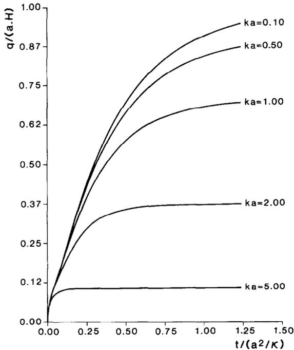
Fig. 5. The heat flow perturbation at time  $t$  after the onset of magma injection in the whole lithosphere at constant rate when the flow is constant at the lower boundary. The heat flow amplitude is  $aH$ . All the other conventions are the same as in Figs. 2 and 3.
