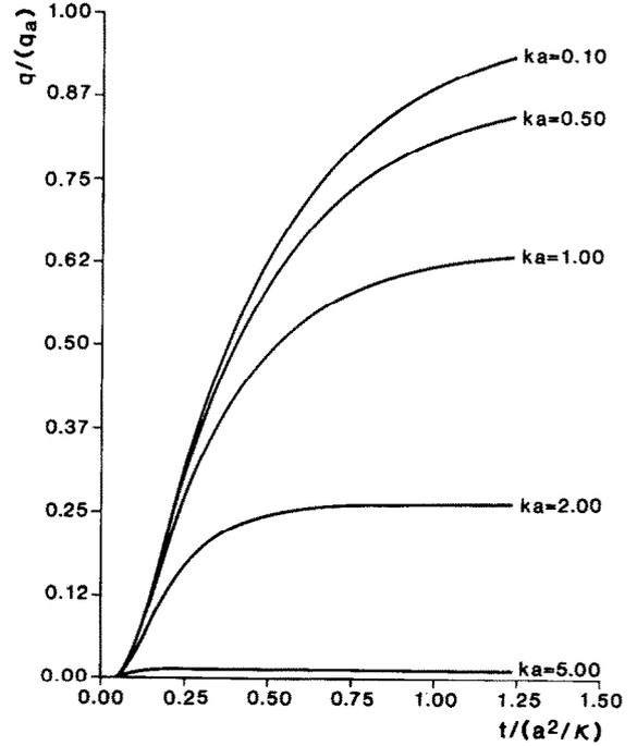
Fig. 2. The surface heat flow at time  $t$  after a stepwise change in heat flow at the lower boundary for different dimensionless wavenumbers (i.e., wavenumber times slab thickness). The time unit is  $a^2/\kappa$ , (300 Ma for the lithosphere, 50 for the crust); the heat flow unit is the amplitude of the lower boundary perturbation.
