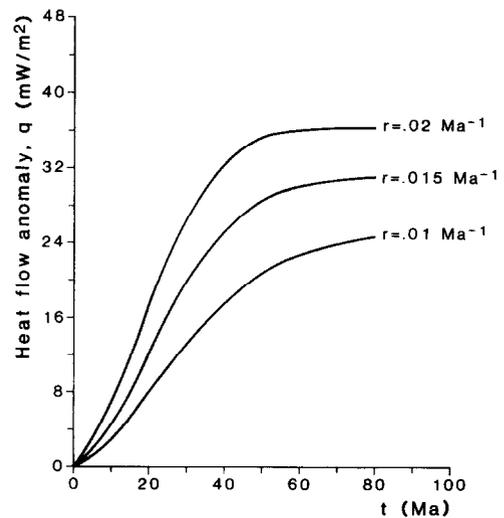
Fig. 9. The surface heat flow as a function of time for the same models when the temperature is constant at the LAB.  $q_m = 20 \text{ mW}/\text{m}^2$ .
