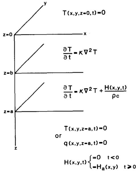
Fig. 4. The geometry, equations, and boundary conditions for the magma injection model.
